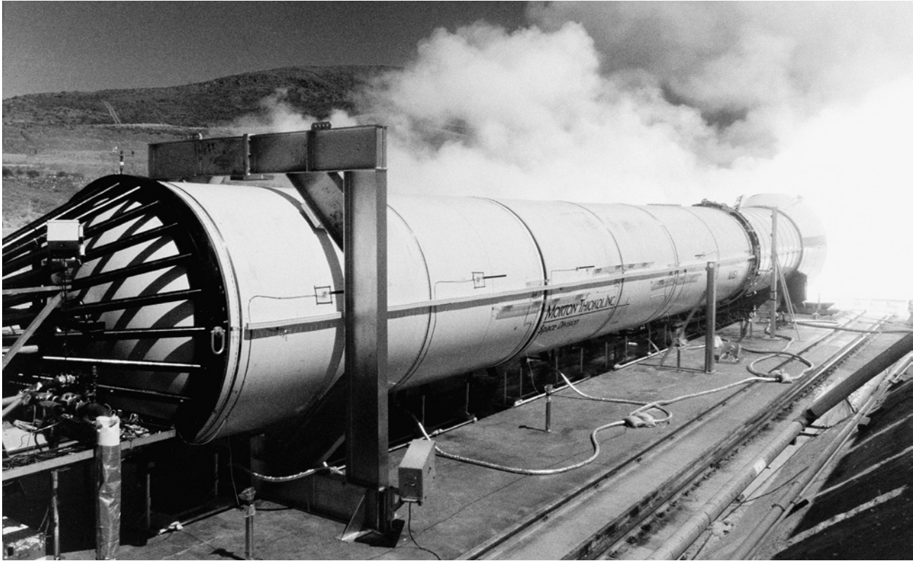
On August 27, 1987, engineers test fire Development Motor-8 at Morton Thiokol's Utah facility. After the explosion of the space shuttle Challenger on January 28, 1986, which was caused by a known problem with the solid rocket boosters that enabled hot gases to bypass two sets of O-ring seals, Morton Thiokol's solid rocket boosters were subjected to a rigorous redesign process and underwent several test firings to recertify them for the new shuttle. The space shuttle Discovery took flight on September 29, 1988.
