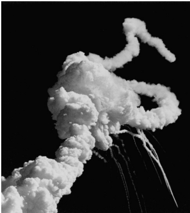
Exhaust plumes from the space shuttle Challenger’s main engines and solid rocket booster entwine around a ball of gas from the external tank a few seconds after the accident, January 28, 1986. An O-ring had ruptured in the right solid rocket booster.
